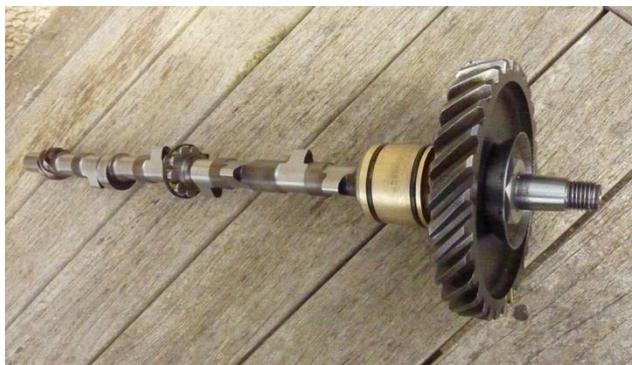
Camshaft assembly ready for insertion
